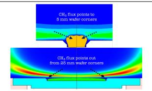
**Fig. 1.** Comparison between 5 mm versus 25 mm diamond growth in a 2.45 GHz reactor highlighting the interplay between the growth rate uniformity and methyl radial distribution.
